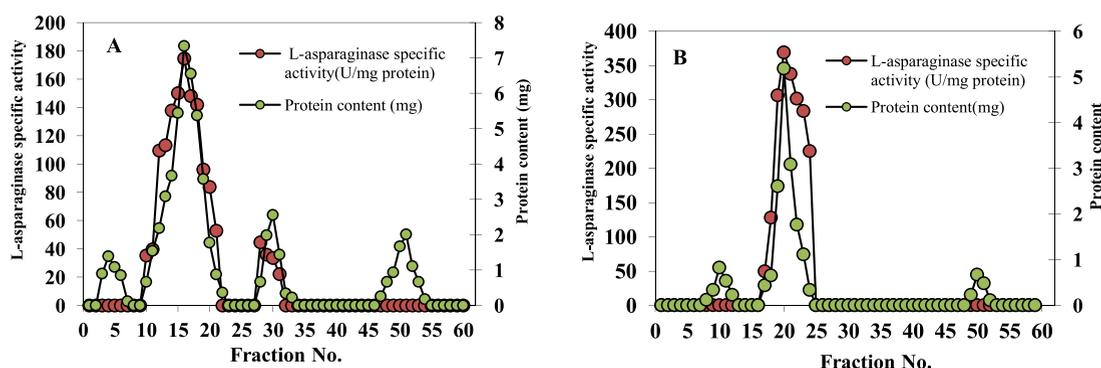
**Fig. 1.** Gel filtration in sephadex-G100 of the semi purified L-asparaginase obtained from *A. terreus* culture (A) and ion-exchange chromatography on DEAE-cellulose of the major active L-asparaginase component obtained from gel filtration (B)
