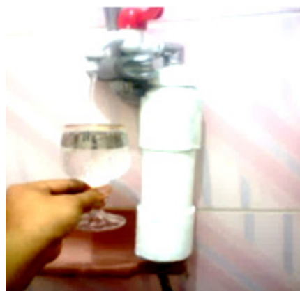
Fig. 1. A designed prototype as a filter column containing the filtration medium for Coliform removal
