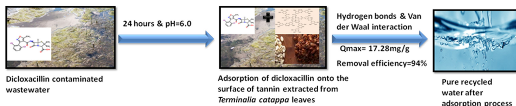
Figure 5. Dicloxacillin adsorption from wastewater by using tannin as bio adsorbent
