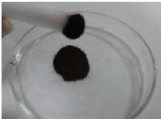
**Fig. 2.** Facile separation of nano-magnetic bacteria bio-composite using external magnetic field
