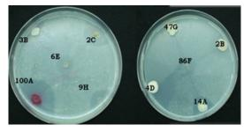
**Fig. 1.** Zone of hydrolysis shown by some isolates on phytase screening medium containing Ca phytate
