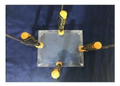
Fig. 1. Silicone poured inside the mold
