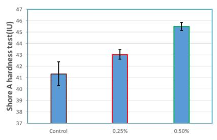
Fig. 10. Bar chart of Shore A hardness represents the mean values and SD from the mean for all study groups
