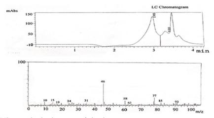
Fig. 16. LCMS reports showing the presence of ethanol
