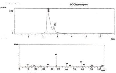
Fig. 15. LCMS reports showing the presence of ethanol
