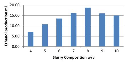
Effect of slurry composition on ethanol production
