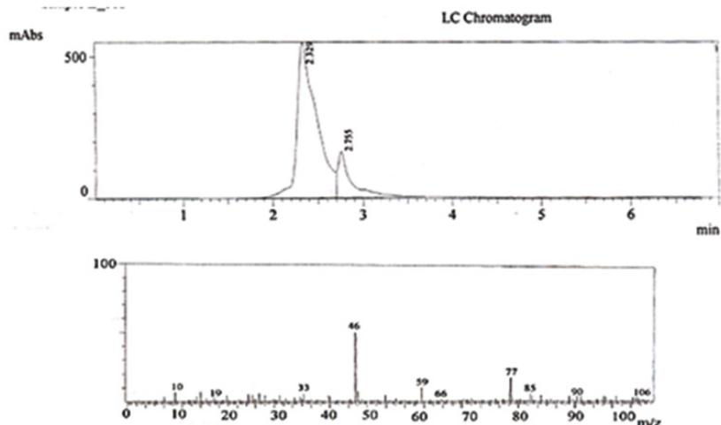
Fig. 15. LCMS reports showing the presence of ethanol
