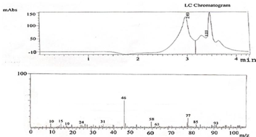
Fig. 16. LCMS reports showing the presence of ethanol
