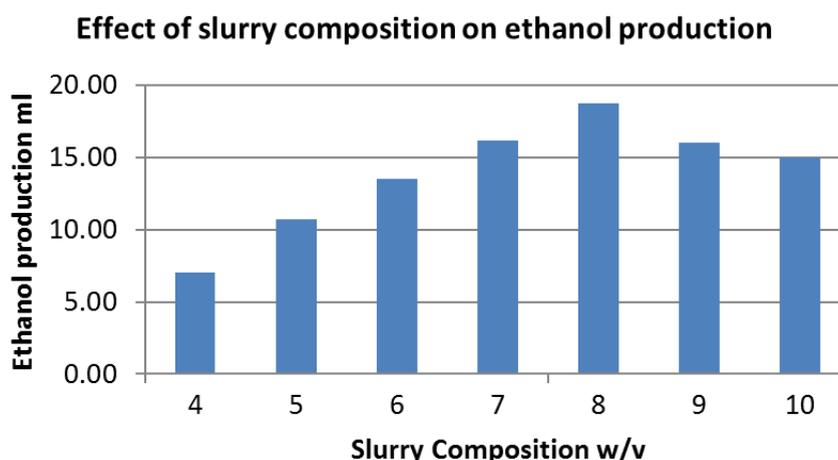
Fig. 1. Effect of slurry composition on ethanol production
