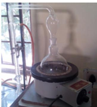
**Fig. 13.** Distillation unit
