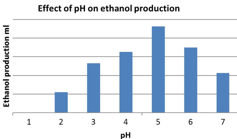
Fig. 2. Effect of pH on ethanol production
