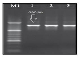
**Fig. 1.** Showed that amplification products of IS711 gene of 696 bp, extracted from B. ovis, Agarose gel electrophoresis of PCR products for IS711 sequence of *Brucella spp*, M1, 50 bp DNA, Ladder, 1-3 well, represented PCR product of *Brucella spp* have 696bp
