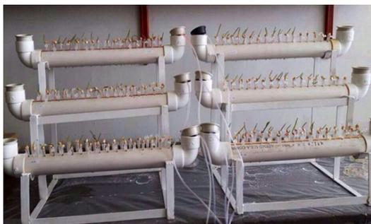
**Fig. 1.** Polyethylene tubes used in the study as hydroponic growth units
