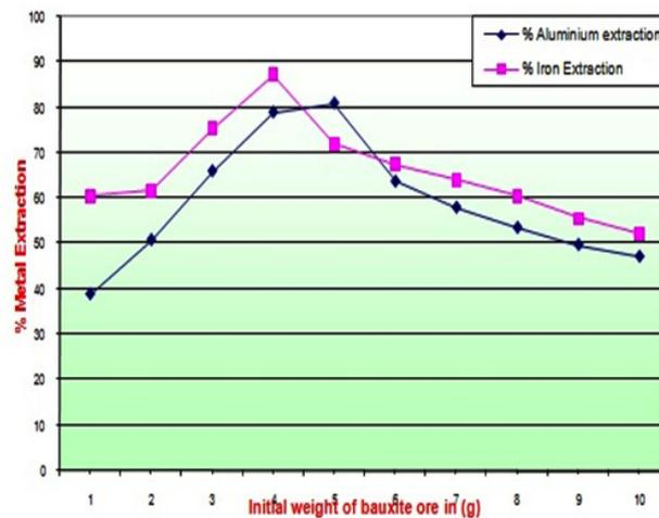
**Graph A.** Effect of pulp density on extraction of metals from bauxite ore by *Acidithiobacillus ferrooxidans*
