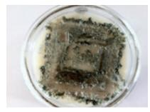
**Plate 1.** Attachment of Dsr2 Strain On Ldpe Sheet (15days)
