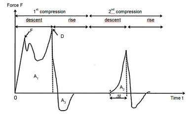
Fig. 2. Typical texture profile after two successive compressions or measurement of TPA "Texture Profile Analysis." Legend: A = surfaces, D = peak forces, "t = time of actual penetration phase during the second compression<sup>11</sup>
