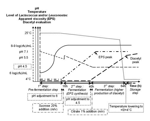
**Fig. 1.** Monitoring of the pre-fermentation, sucrose and citrate fermentation steps for EPS and diacetyl production by respectively EPS positive *Leuconostoc* strain (P35) and citrate positive *Lactococcus* strain (F2.3). The actions written in boxes were those performed to guide the fermentation process.
