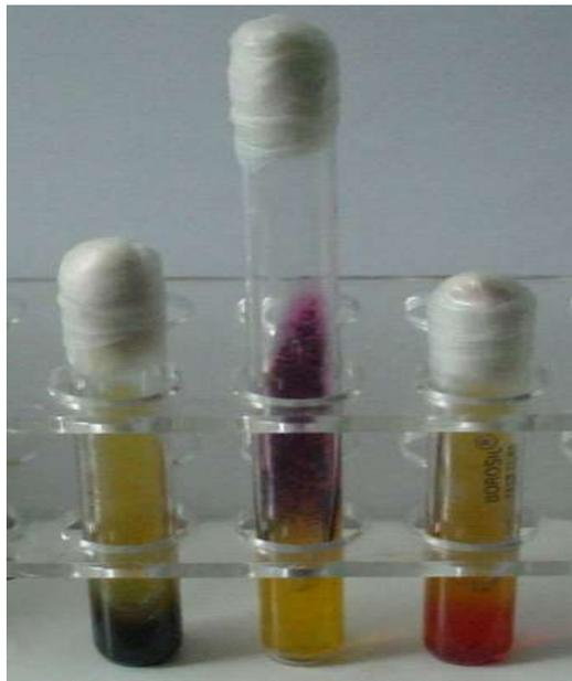
**Fig. 1.** TSI test showing positive hydrogen sulphide gas and glucose fermentation
