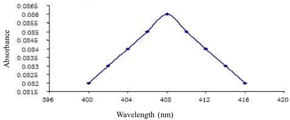
Fig. 3. Absorption spectra of procion yellow
