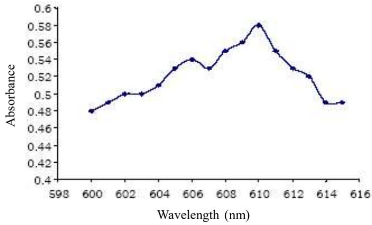
Fig. 1. Absorption spectra of procion navy blue
