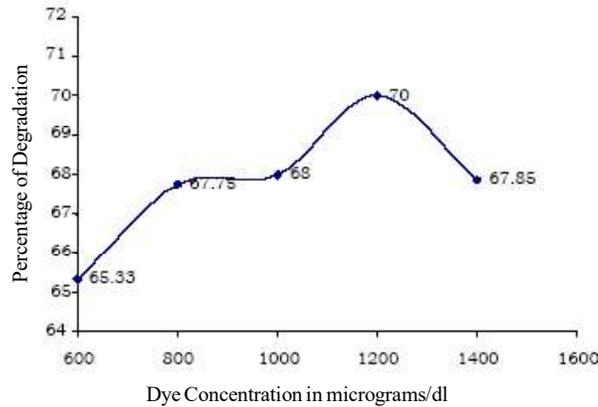
Fig. 5. Optimization of dye concentration for procion brilliant red degradation
