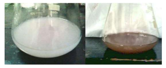
(a) Pale white color observed immediately after exposure of fungal biomass to 1mM AgNO<sub>3</sub>
