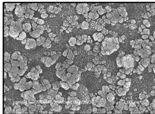
**Fig. 3.** SEM micrograph of Ag nanoparticles formed by *Fusarium oxysporum*
