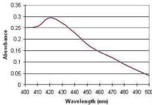
**Fig. 2.** Detection of Ag nanoparticles through UV-visible spectroscopy
