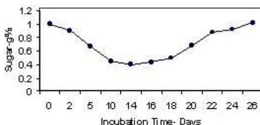
Fig. 3. Variation of sugar concentration during the growth of Trichoderma viride in presence of hardwood sawdust
