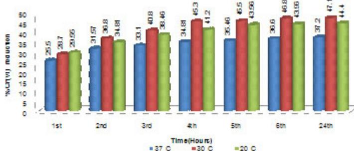
Fig. 3. Hexavalent chromium reduction by *A. calcoaceticus* in PBS at different temperatures
