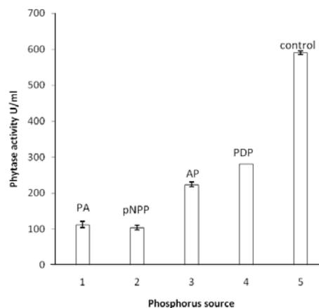
**Fig. 8.** Effect of different phosphorus source on phytase production. PA-potassium nitrate, pNPP-para nitrophenyl phosphate, AP-Ammonium phosphate, PDP-potassium dihydrogen phosphate, control – without any phosphate source
