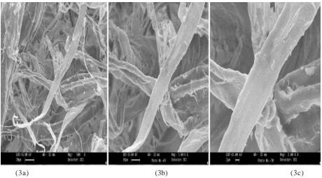
**Fig. 3**. Scanning electron micrograph of enzymatic deinked old news paper pulp at 500X (3a), 1000X (3b) and 2000X (3c) respectively
