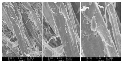
(2a) (2b) (2c) **Fig. 2**. Scanning electron micrograph of chemical deinked old newspaper pulp at 500X(2a), 1000X (2b) and 2000X (2c) respectively
