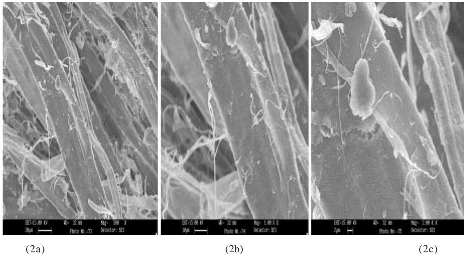
**Fig. 2.** Scanning electron micrograph of chemical deinked old newspaper pulp at 500X(2a), 1000X (2b) and 2000X (2c) respectively
