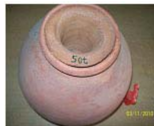
Filtration system 50T inserted in the receiving pot
