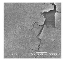
B) Disc Surface after Degradation
