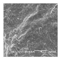
A) Disc Surface before Degradation
