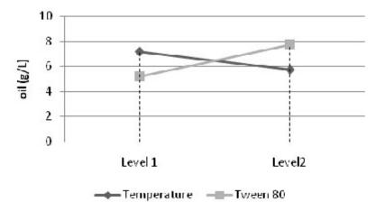
Fig. 4. Main effect of two level factors on oil production
