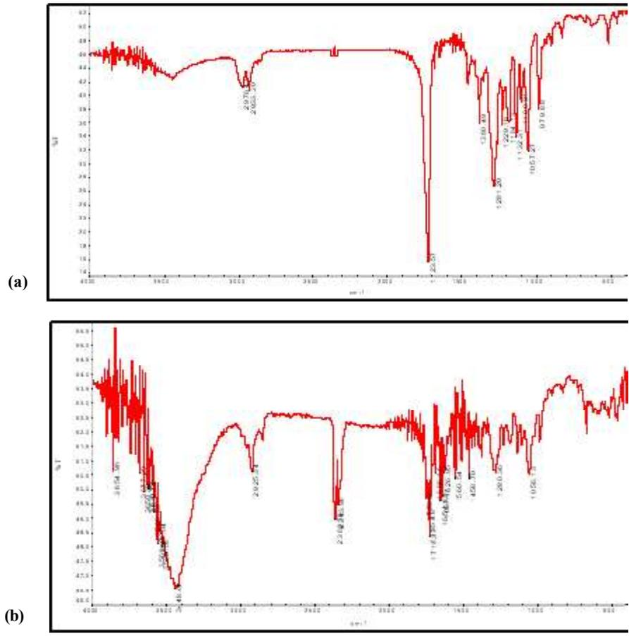
Fig. 4. FTIR of PHB purified from *Haloarcula* sp. 1 AB 19 (a) Standard (b) Sample
