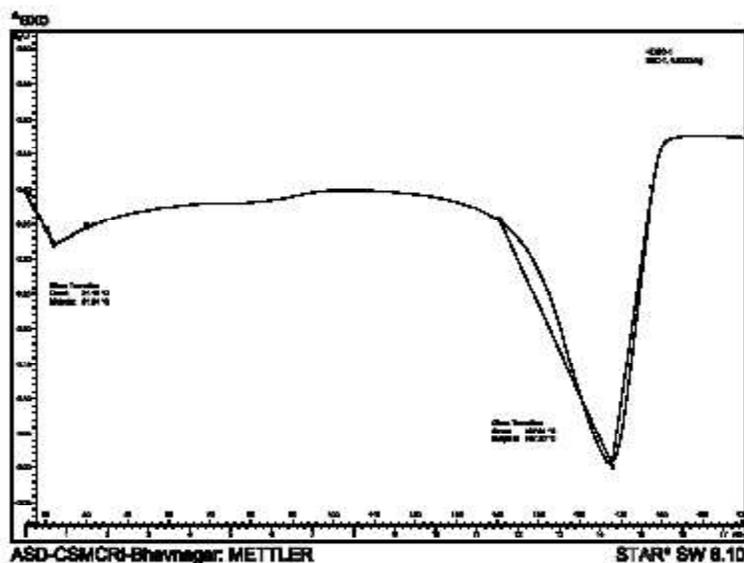
Fig. 7. DSC thermogram of PHB produced from *Haloarcula* sp. AB 19
