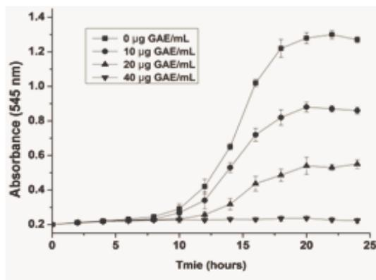
Fig. 2. Growth curves of *B. subtilis* measured by UV-Vis spectroscopy at 545 nm at different time intervals
