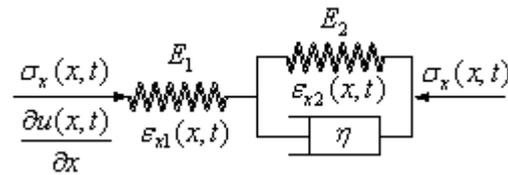
Fig. 2. Three-parameter solid of *N*-layered CNTs
