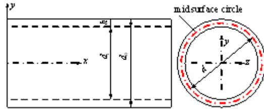
Fig. 1. Layout of *N*-layered CNTs.
