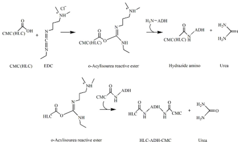
**Fig. 2.** Scheme of the cross-linking processes. The HLC, CMC or ADH in the figure are represented as complete molecules except for the reacted carboxylic group or amino group
