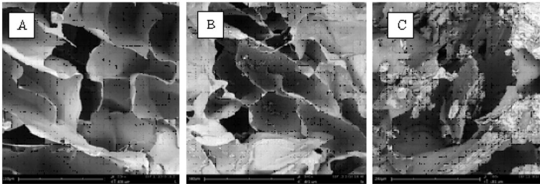
**Fig. 1.** SEM micrographs (x500) of CMC-HLC/EDC-ADH hydrogels at 37 °C after lyophilization (A), after degradation by collagenase I (B), after SBF degradation (C)
