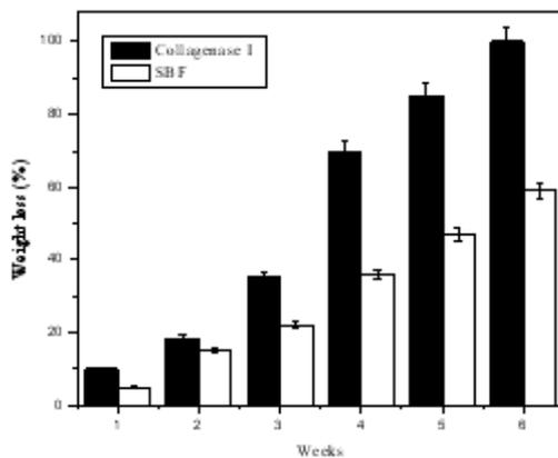
Fig. 4. The weight loss of hydrogels degradation by collagenase I and SBF
