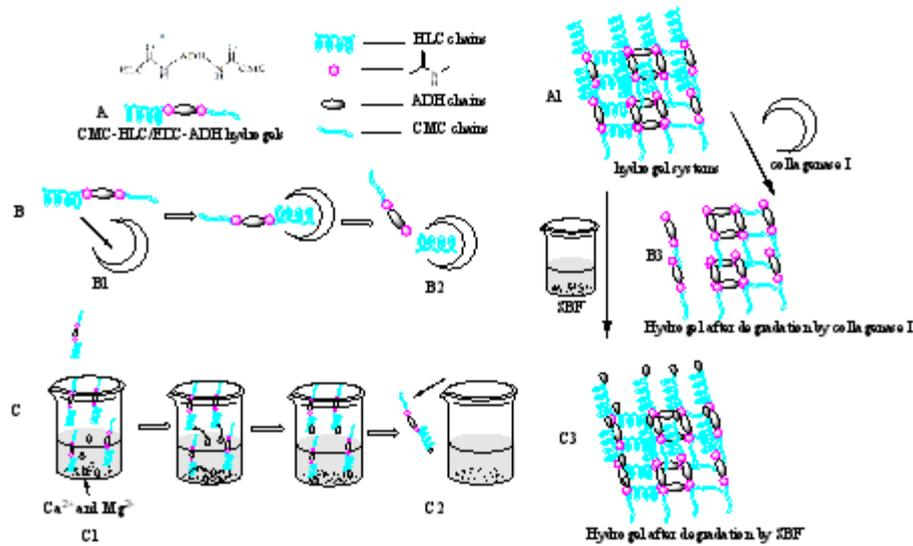
Fig. 3. Scheme of the degradation by collagenase I and SBF
