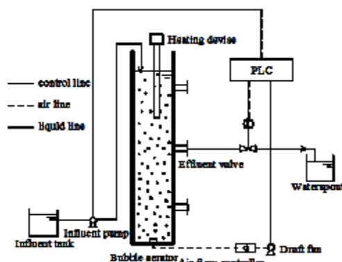
Fig. 1. Schematic diagram of SBR installation
