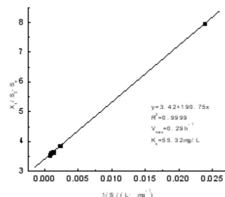
**Fig. 6.** Degradation dynamics of activated sludge
