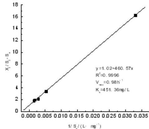
**Fig. 5.** Degradation dynamics of aerobic granular sludge.
