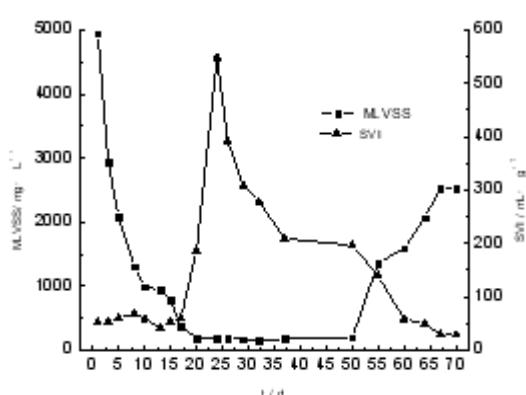
**Fig. 3.** Variations of MLVSS and SVI during the operation
