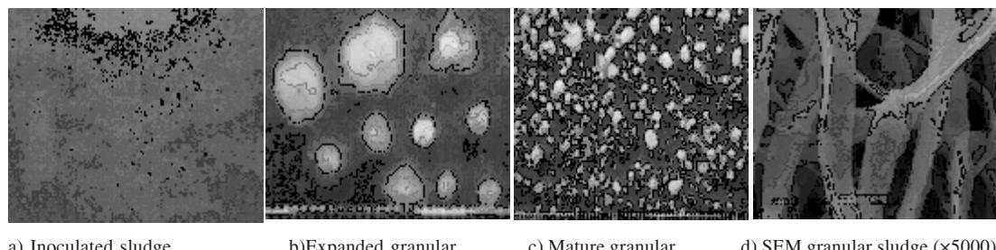
**Fig. 2.** Variations of granule sludge image in different training times
