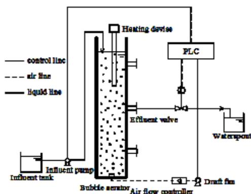
Fig. 1. Schematic diagram of SBR installation
