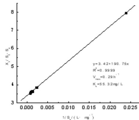
**Fig. 6.** Degradation dynamics of activated sludge
