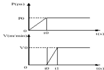
**Fig. 2.** Pressure and Material Extrusion Velocity with Time
