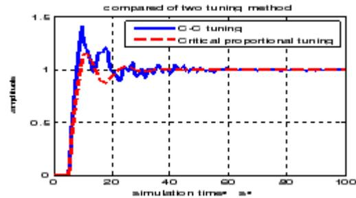
Fig. 3. Step Response of Tuning Methods
