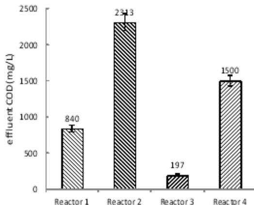
**Fig. 3.** Effluent COD of the four reactors
