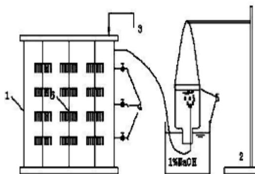
1-ASBBR reactor 2-bracket 3-intake 4-sampling ports
