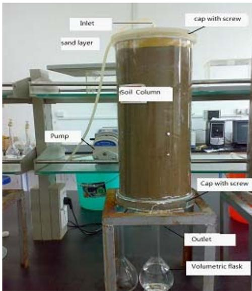
Fig. 1. Experiment set up for measuring solute flow through an undisturbed silt loam soil column
