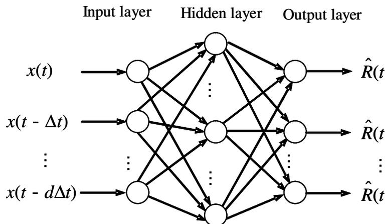
Fig. 1. The model structure of reliability prediction based on BPNN
