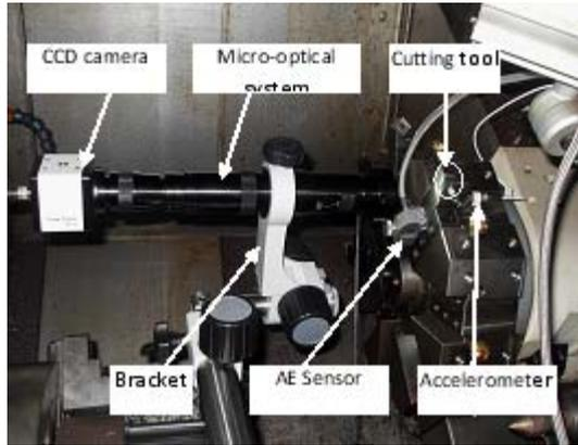
Fig. 2. The installation of micro-optical system accelerometer and AE sensor
