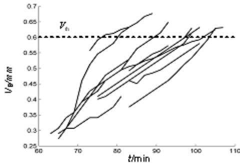
Fig. 3. Time-varying wear data of the tools
