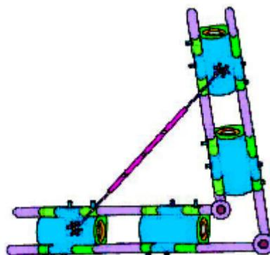
Fig. 3. Minimum djustment angle (60 degree)
