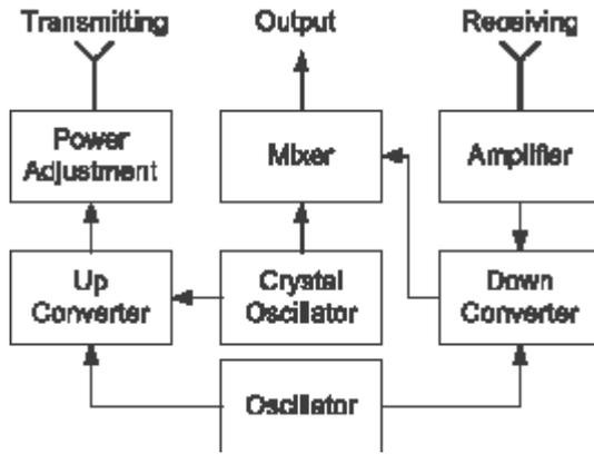
Fig. 1. Schematic diagram of the bioradar speech-detection system
