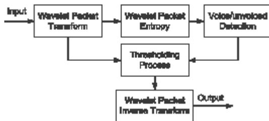
Fig. 2. The proposed adaptive wavelet packet entropy speech enhancement algorithm
