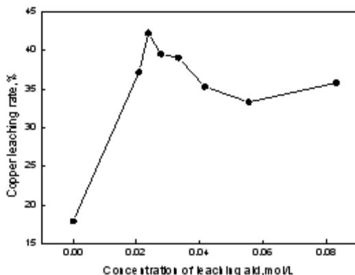
Fig. 5. Effect of leaching aid concentration on copper leaching rate
