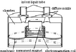
Fig. 1. A perspective view of the electromagnetic micropump
