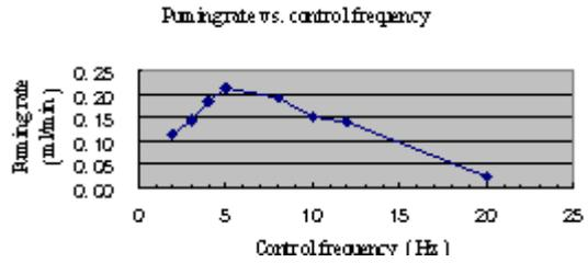
Fig. 4. Pumping rate vs. control frequency
