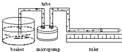
Fig. 3. The test and measurement setup
