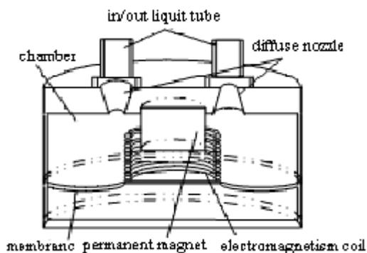
Fig. 1. A perspective view of the electromagnetic micropump
