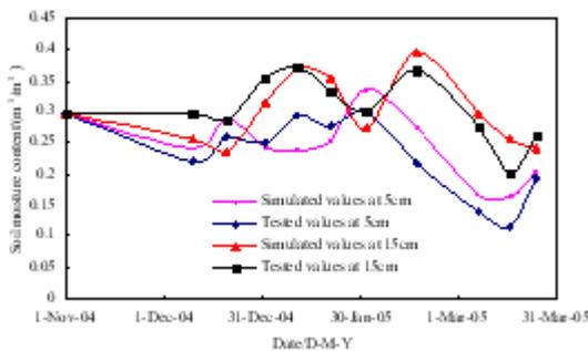
Fig. 3. Comparison between the simulated and tested soil moisture content at 5cm and 15cm
