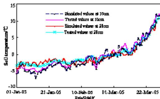
**Fig. 5.** Comparison between the simulated and tested soil temperature at 10 cm and 20 cm
