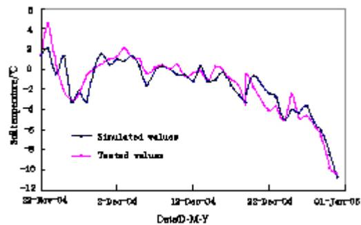
Fig. 2. Comparison between simulated and tested surface soil temperature
