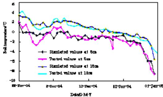
Fig. 1. Comparison between simulated and tested soil temperature at 5cm and 15cm
