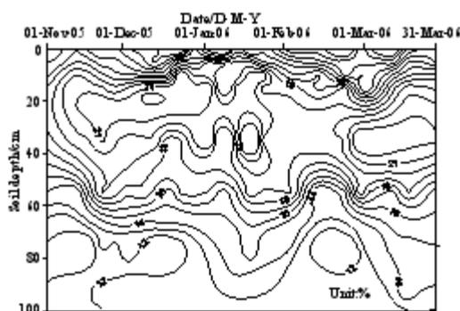
Fig. 7. Soil moisture content isograms of bare plot
