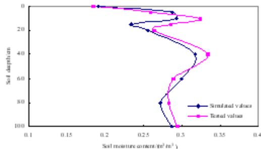
Fig. 4. Comparison between the simulated and tested soil moisture content on December 20, 2004
