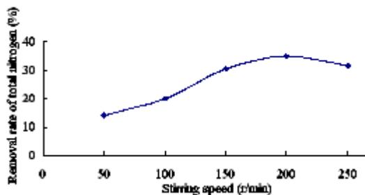
Fig. 4. Removal rate of total nitrogen with different stirring speed
