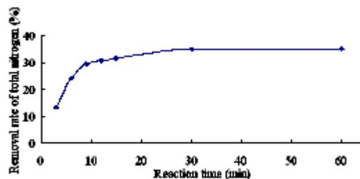
Fig. 5. Removal rate of total nitrogen with different reaction time
