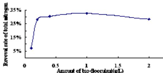
Fig. 3. Removal rate of total nitrogen with different amount of bioflocculant
