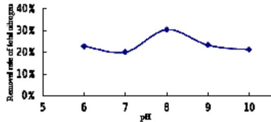
Fig. 1. Removal rate of total nitrogen at different pH
