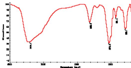
Fig. 6. Fourier transform infrared spectrum for the prepared bioflocculant
