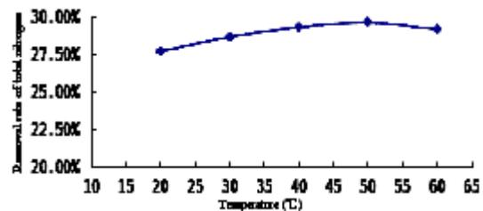
Fig. 2. Removal rate of total nitrogen at different temperature
