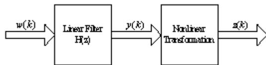
Fig. 2. Block diagram of the clutter modeling of ZMNL method
