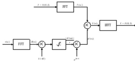
Fig. 3. Principle diagram of generating relevant Gaussian sequence
