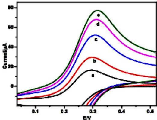
Fig. 5. Cyclic voltammograms of Ag-RGO modified GCE electrode with various scan rate: (a) 10, (b) 20, (c) 50, (d) 80, and (e) 100 mV/s; Inset: plots of peak current ( $I_p$ ) against square root of the scan rates ( $v^{1/2}$ )
