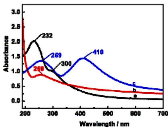
Fig. 1. UV-Vis absorption spectra of (a) GO, (b) RGO, and (c) Ag-RGO hybrid; insets: a photograph of GO (left), RGO (middle) and Ag-RGO (right) composite solutions
