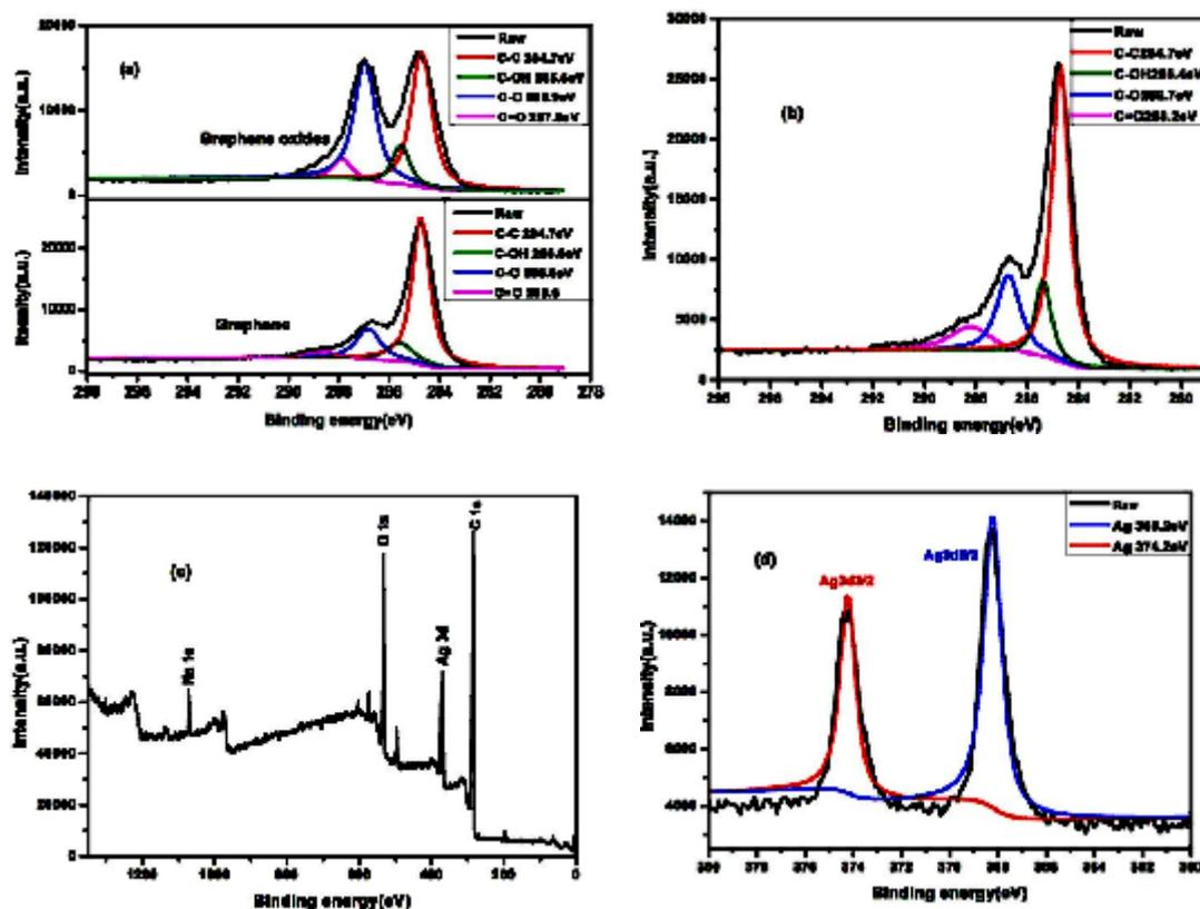
Fig. 2. C 1s XPS spectra of (a) GO and RGO, (b) Ag-RGO; XPS spectra of the Ag-RGO nanocomposites (c), and the Ag 3d doublet (d)
