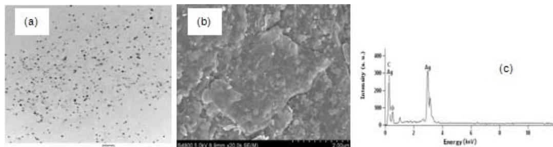
Fig. 3 (a) TEM image, (b) SEM image and (c) EDX analysis of Ag-RGO nanocomposites
