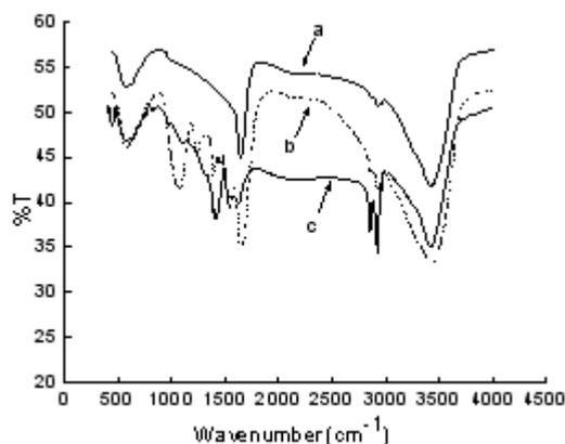
Fig. 2. FT- IR spectra of MNPs a, carboxyl-functionalized MNPs; b, *Aeromonas* sp. F3 loaded with MNPs; c, pure MNPs
