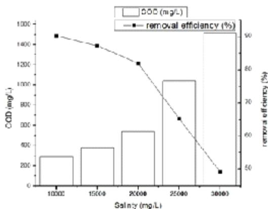
Fig. 2. COD and removal efficiency at different salinity
