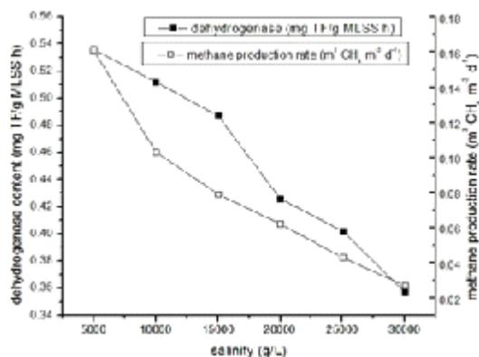
Fig. 3. Dehydrogenase content and CH<sub>4</sub> production rate at different salinity
