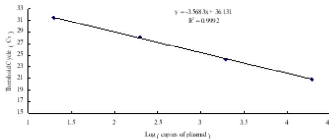
**Fig. 2.** Standard curve based on plasmid with the varying copies ( $1.94 \times 10^4 \sim 1.94$  copies  $ul^{-1}$ ) plotted vs the cycle threshold (C<sub>T</sub>) values
