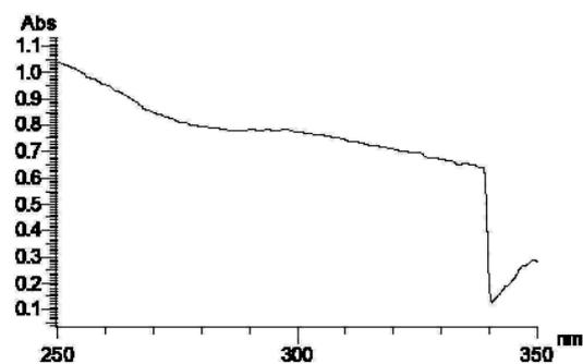
Fig. 1. UV-visible absorption spectra of the ZnO nanoparticles
