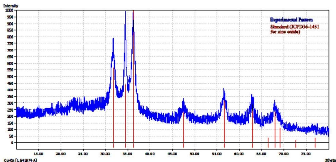
Fig. 2. X-ray diffraction pattern of ZnO particle in powdered form.
